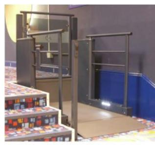
Wait for the ramp to fully lower, it is now safe to exit the lift.
